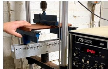
Ludowici regularly completes ASTM C 1167 - Quality Assurance breaking-strength tests on clay tiles manufactured for projects like University of Chicago’s Classic 14” Interlocking profile.
