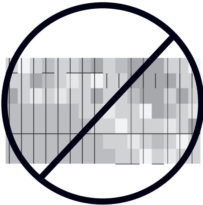
Figure 24.2 Improperly Blended Spanish Tile. There Should Be No Hotspots or Diagonal Patterns Visible.
