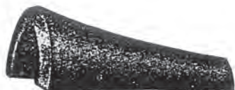
H. - 11 HIP ROLL Length ..... 14\frac{1}{2} ins. Exposure ..... 12 ins. Span, inside ..... 6 ins. Height ..... 5 lbs. Weight, per ft., 5\frac{1}{2} lbs.
