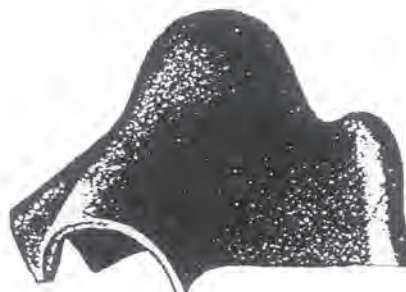
No. 405 Base width ..... 14 ins. Top width ..... 5 ins. Total height ..... 14 ins. Weight ..... 5 lbs. Two-way Hipped Terminal for Crestings No. 213 or 303, and Hip Rolls No. 109 or 113.
