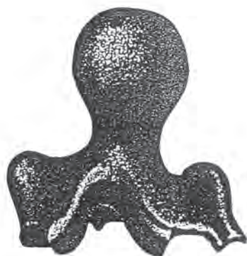
No. 415 Base width ..... 19 ins. Height ..... 20 ins. Ball diameter .... 10 ins. Weight ..... 37 lbs. Two-way Terminal for use with Cresting No. 210 and Hip Roll No. 104.
