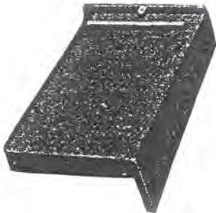
RIGHT WIDE GABLE RAKE Depth of flange below sheathing, one inch. Weight, per ft., 7½ lbs.
